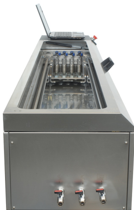
Detail of the ductilometer's test area with frame and tank all stainless steel made
